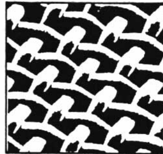
Monofilament Polyester mesh is made from single strands of polyester.
