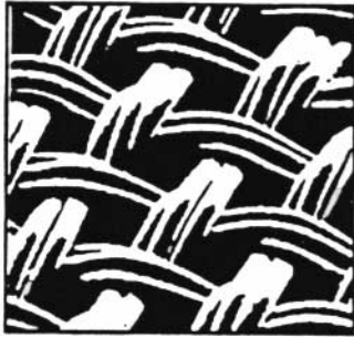
Multifilament Polyester mesh is made from twisted strands of polyester
